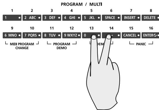
A label below the 13 & 14 Program/Multi buttons indicates the Demo double button press.
